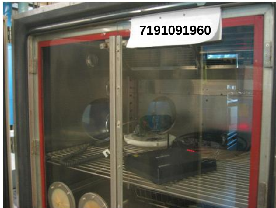
Frequency Stability (Temperature Variation) Test Setup
