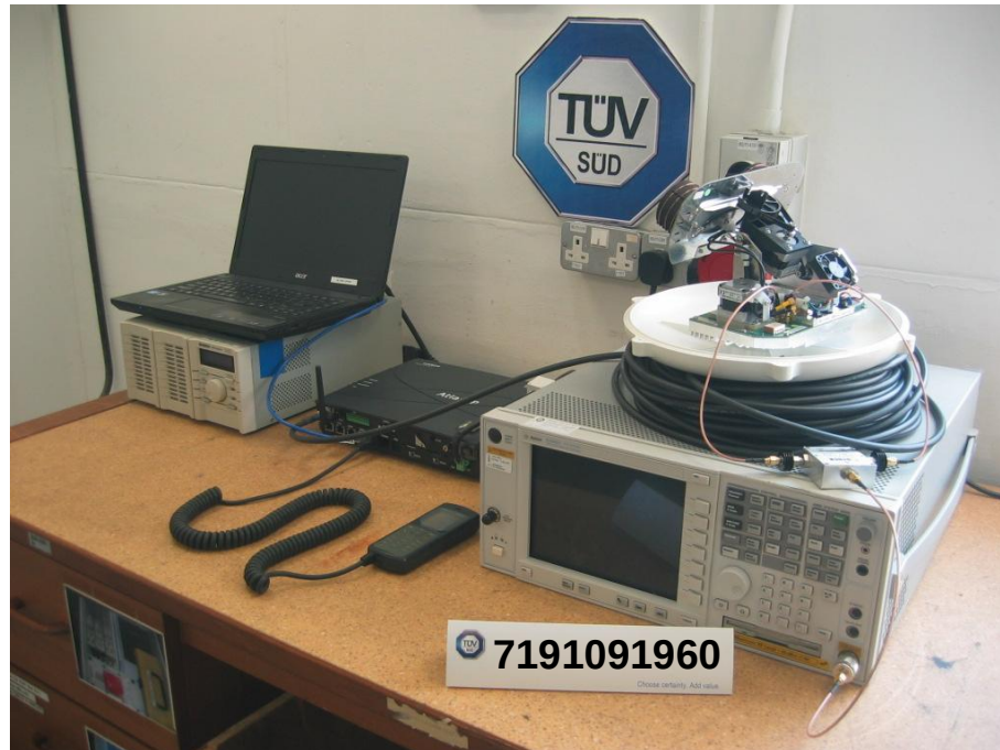
RF Output Power Test Setup
