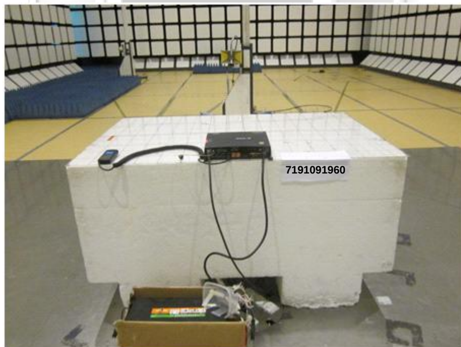
Radiated Emissions Test Setup (Rear View)
