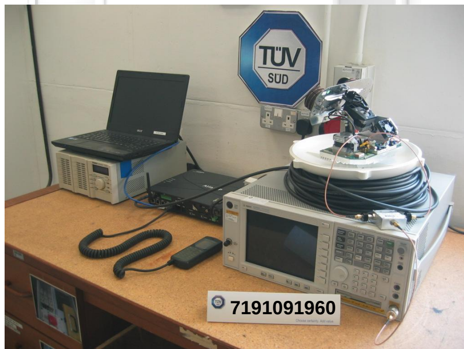
Unwanted Emissions at Antenna Terminal Test Setup
