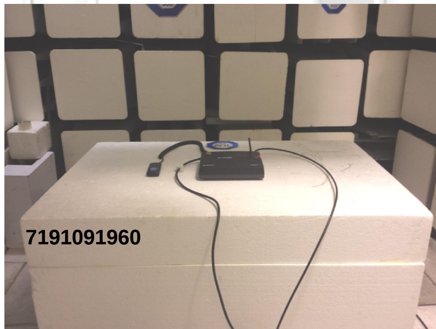
Radiated Spurious Emissions Test Setup (Rear View)
