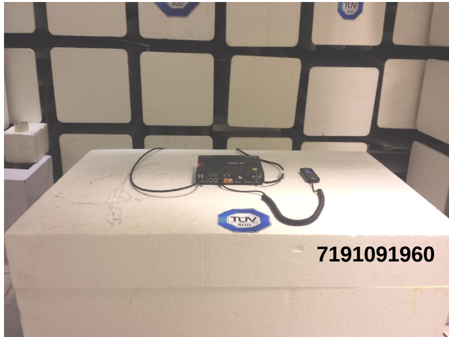
Radiated Spurious Emissions Test Setup (Front View)
