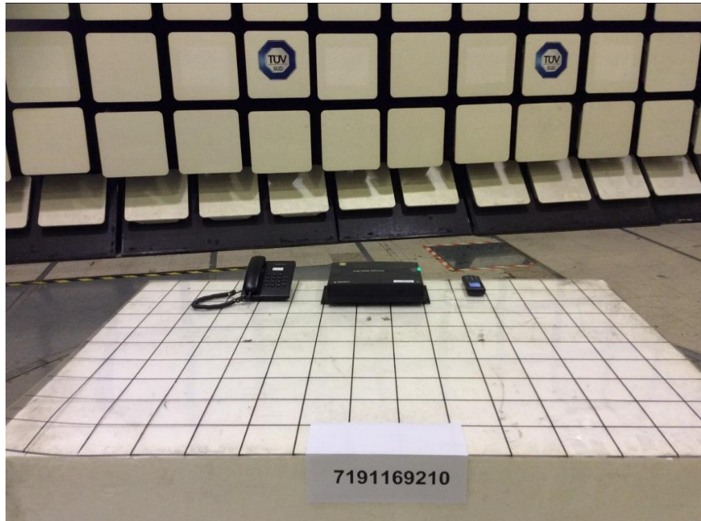
Radiated Emissions & Radiated Spurious Emissions Test Setup (Front View)
