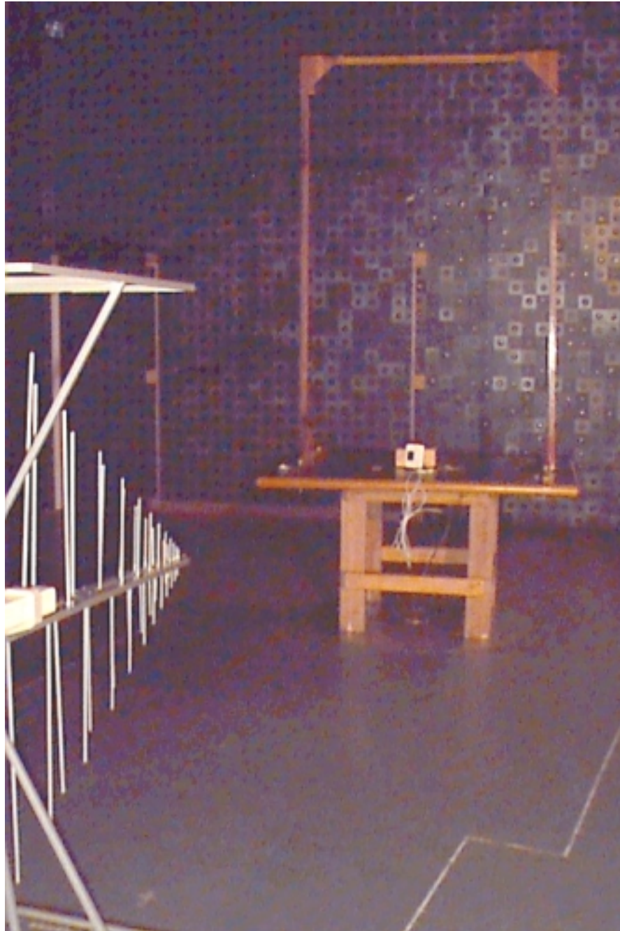
Photograph 2 Radiated emission measurements test setup with biconilog antenna, 30 MHz – 1000 MHz frequency range, anechoic chamber method
