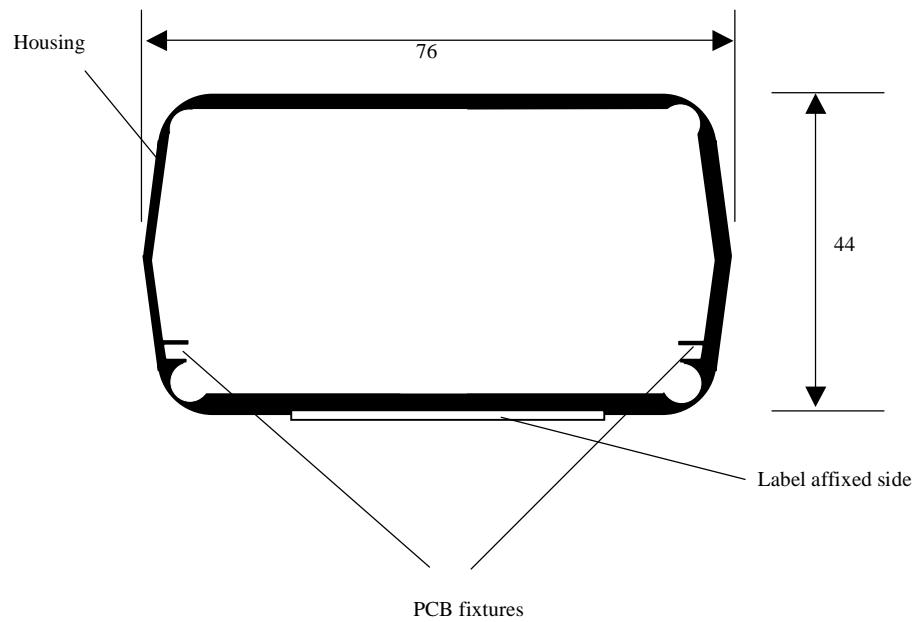
All dimensions are in mm with tolerance +/- 0.5mm.
