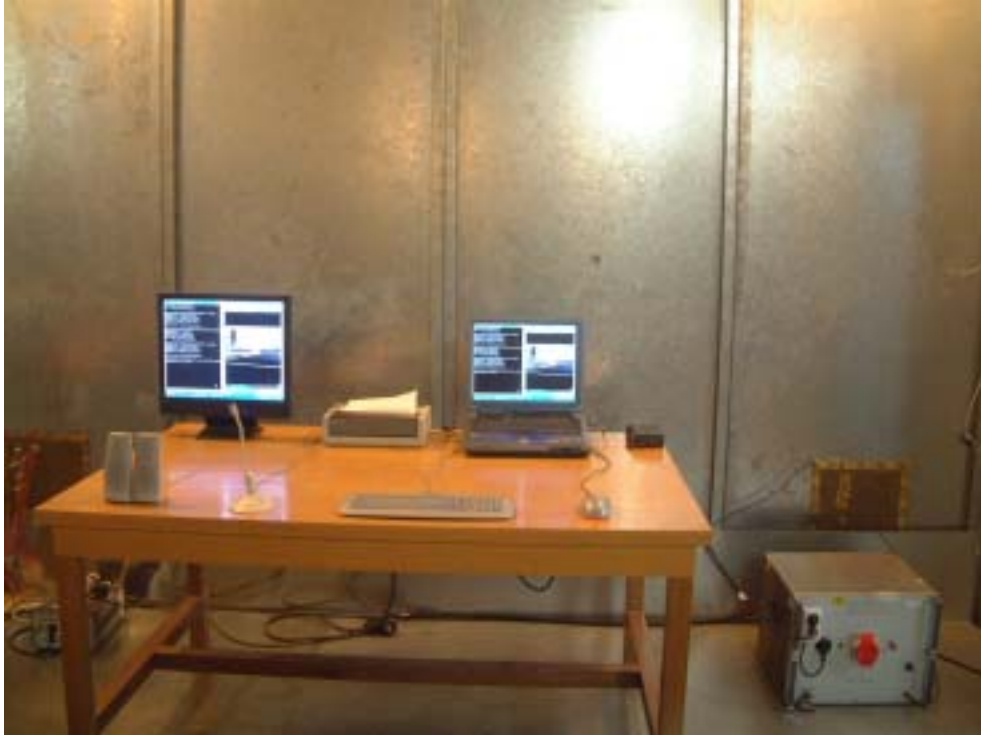
LINE CONDUCTED SETUP PHOTOGRAPH - FRONT VIEW
