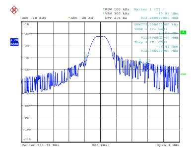
Low Channel (911.78 MHz) 99% Occupied Bandwidth is 772 kHz
