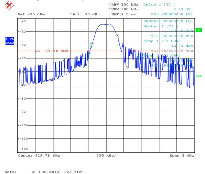
High Channel (919.78 MHz) 99% Occupied Bandwidth is 588 kHz
