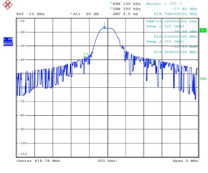
High Channel (918.78 kHz) 99% Occupied Bandwidth is 732 kHz
