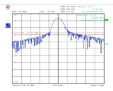
High Channel (918.78 kHz) 20dB Occupied Bandwidth is 512kHz
