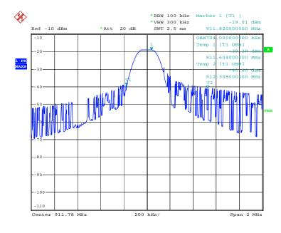
Low Channel (911.78 kHz) 99% Occupied Bandwidth is 704 kHz
