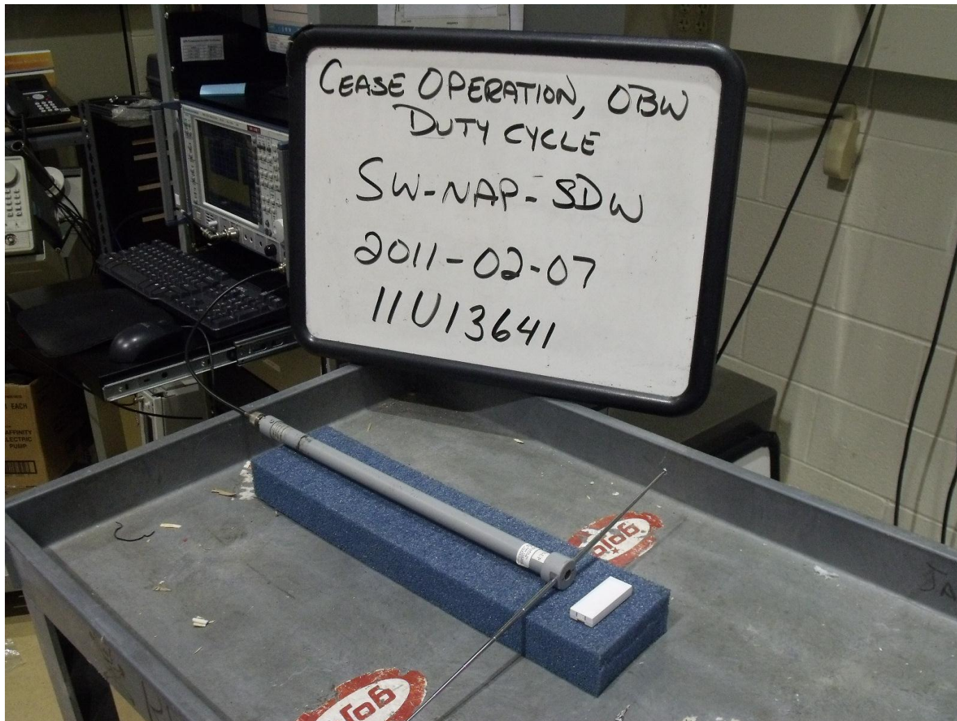
Figure 1 Test Setup for Occupied Bandwidth
