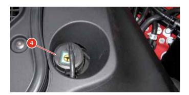
Top up if necessary with the recommended oil up to the  $\mbox{\bf MAX}$  reference mark.
