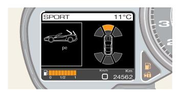
For the repainting of bumpers or retouching the paintwork in the sensor area, contact the Ferrari Service Network. If paint is applied incorrectly, it may jeopardise proper operation of the parking sensors.
