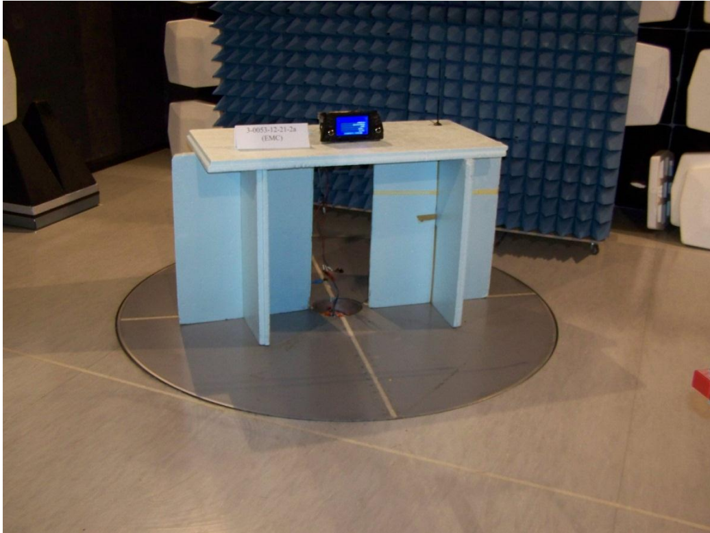
Photograph 3: Radiated measurements test set-up (Semi-Anechoic-Chamber)
