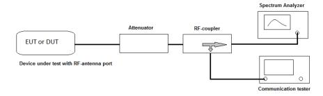
**Testing method:** According to ANSI 63.10-2009 for each individual test, see more details in each
