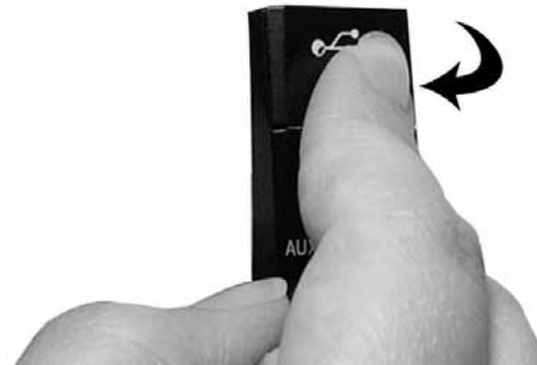
3. Then push on the bottom of the flap to secure in place.
