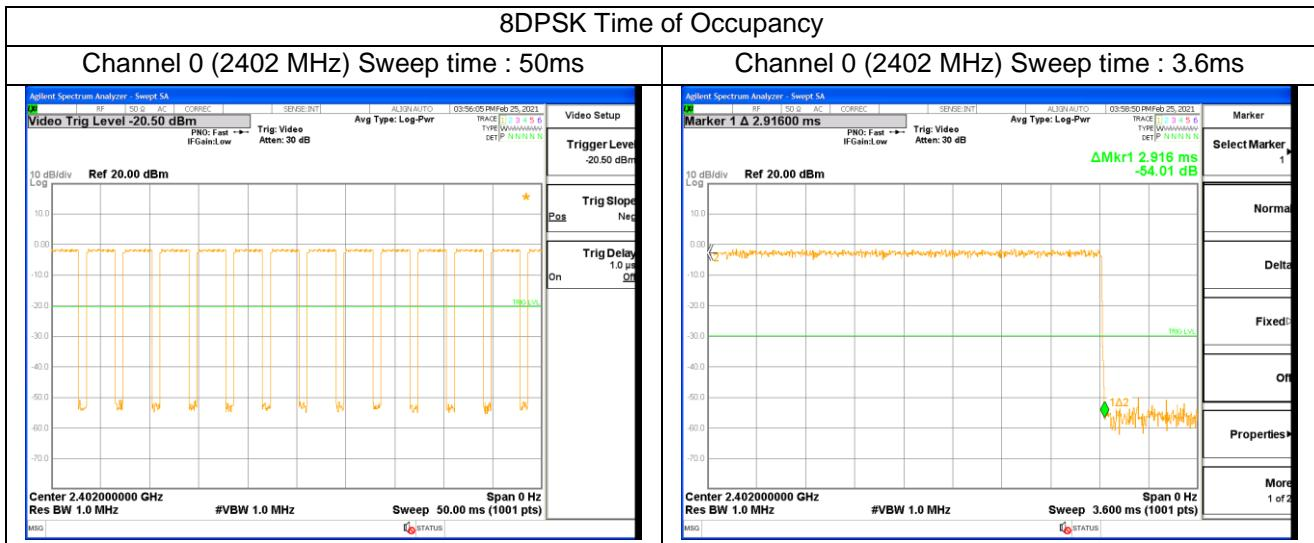
Note : Test Time Period:  $0.4 * 79 = 31.6$ sec, Hopping Time with 1sec :  $14/50\text{ms} = 280$  hops/sec.
