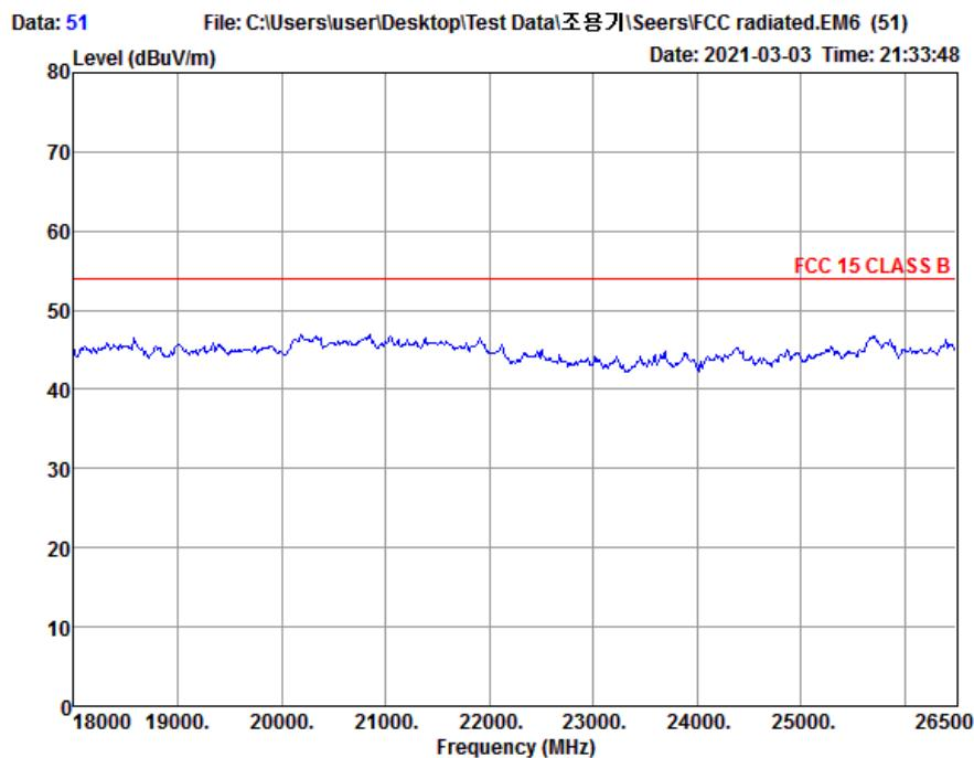
Note <sup>(1)</sup> : Only the worst case plots for Radiated Spurious Emissions.Note <sup>(2)</sup> : No other emissions were detected.
