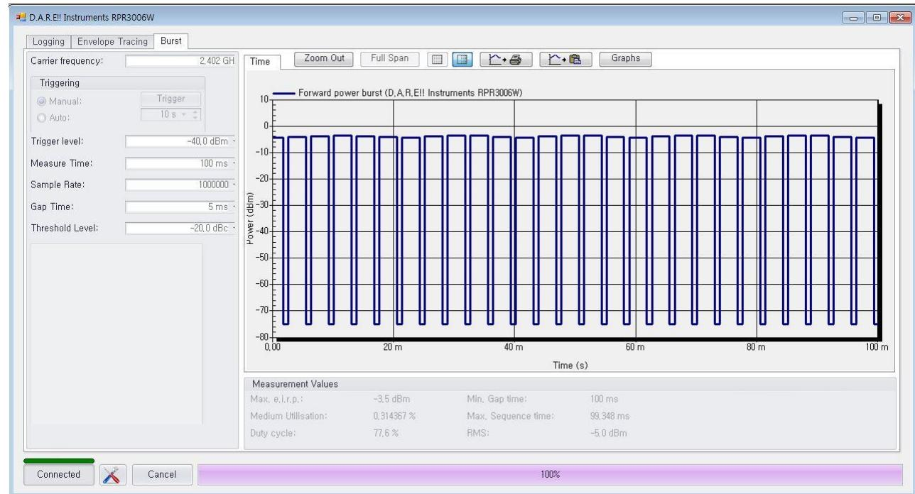
Test Mode : EDR( $\pi/4$ -DQPSK) 2441 MHz
