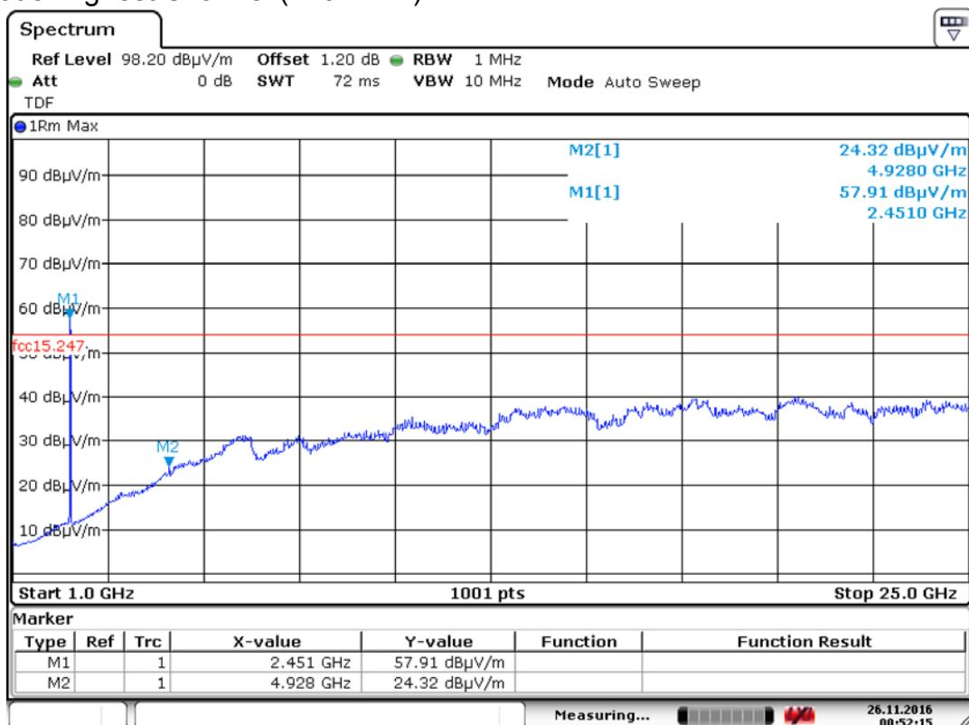
**[Radiated Band Edges Test]****The Test result is record to the worst case test data.**
