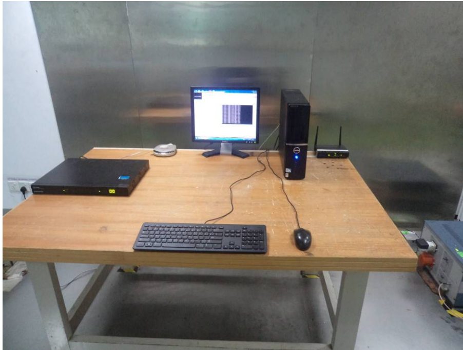
AC Line Conducted Emissions – Front View
