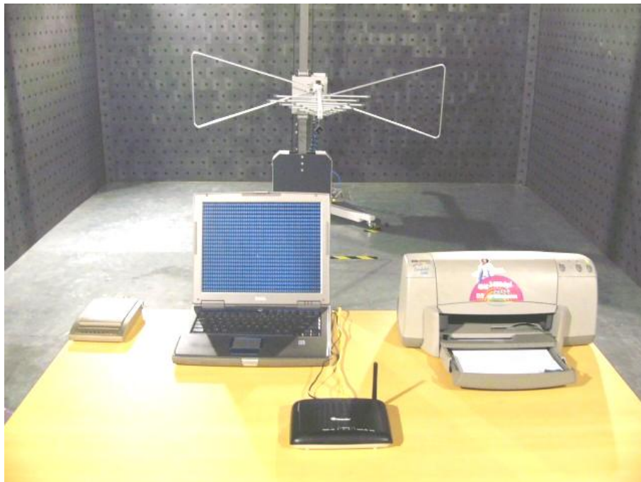
Radiated emission test view
