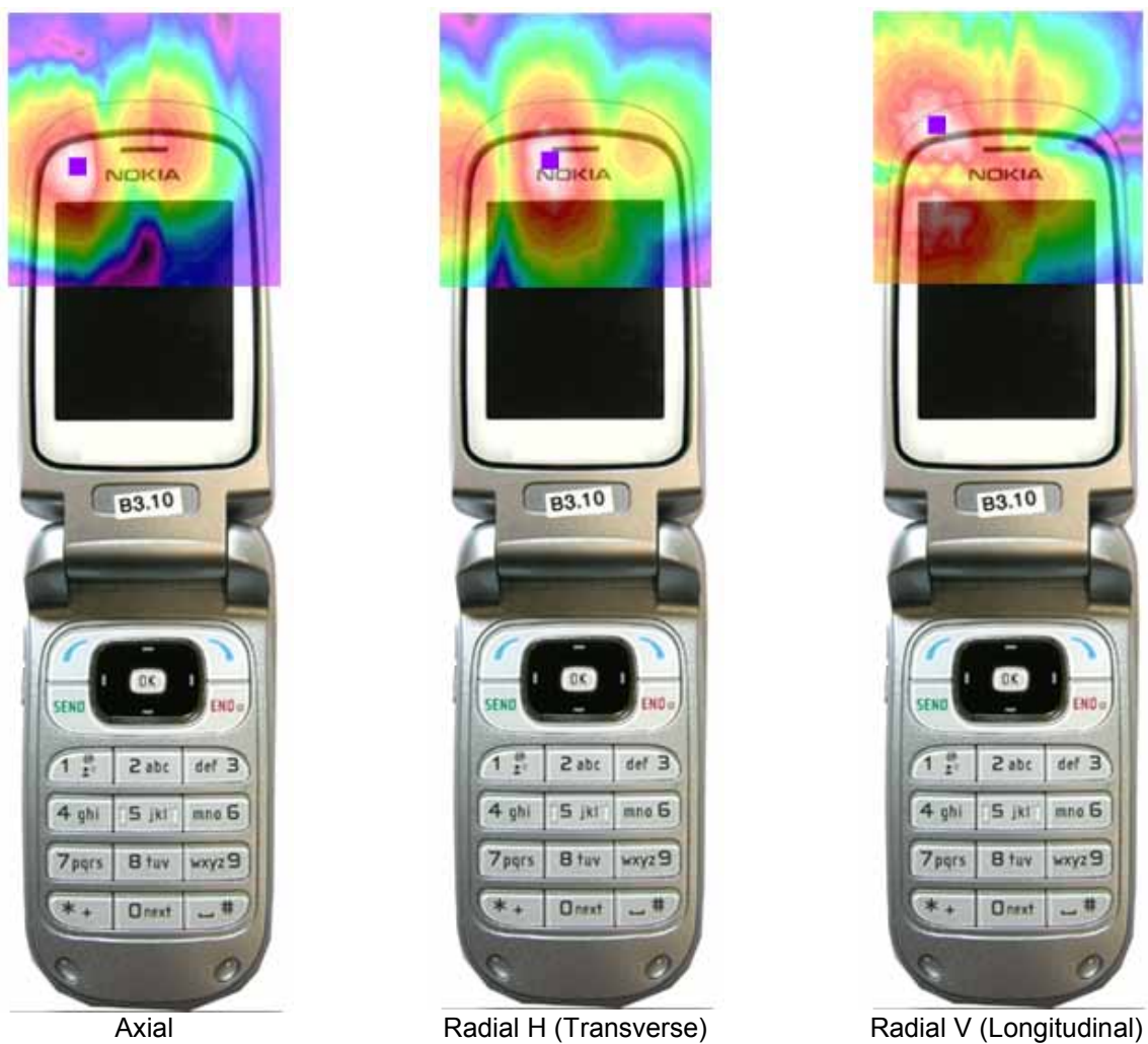
Figure 13-3 T-Coil Scan Overlay Magnetic Field Distributions
