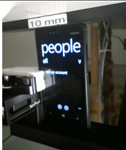
Photo of the device positioned for WR mode measurement – top edge facing phantom. The spacer was removed before the start of the measurements.
