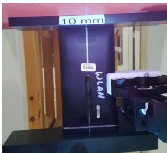
Photo of the device positioned for WR mode measurement – bottom edge facing phantom. The spacer was removed before the start of the measurements.
