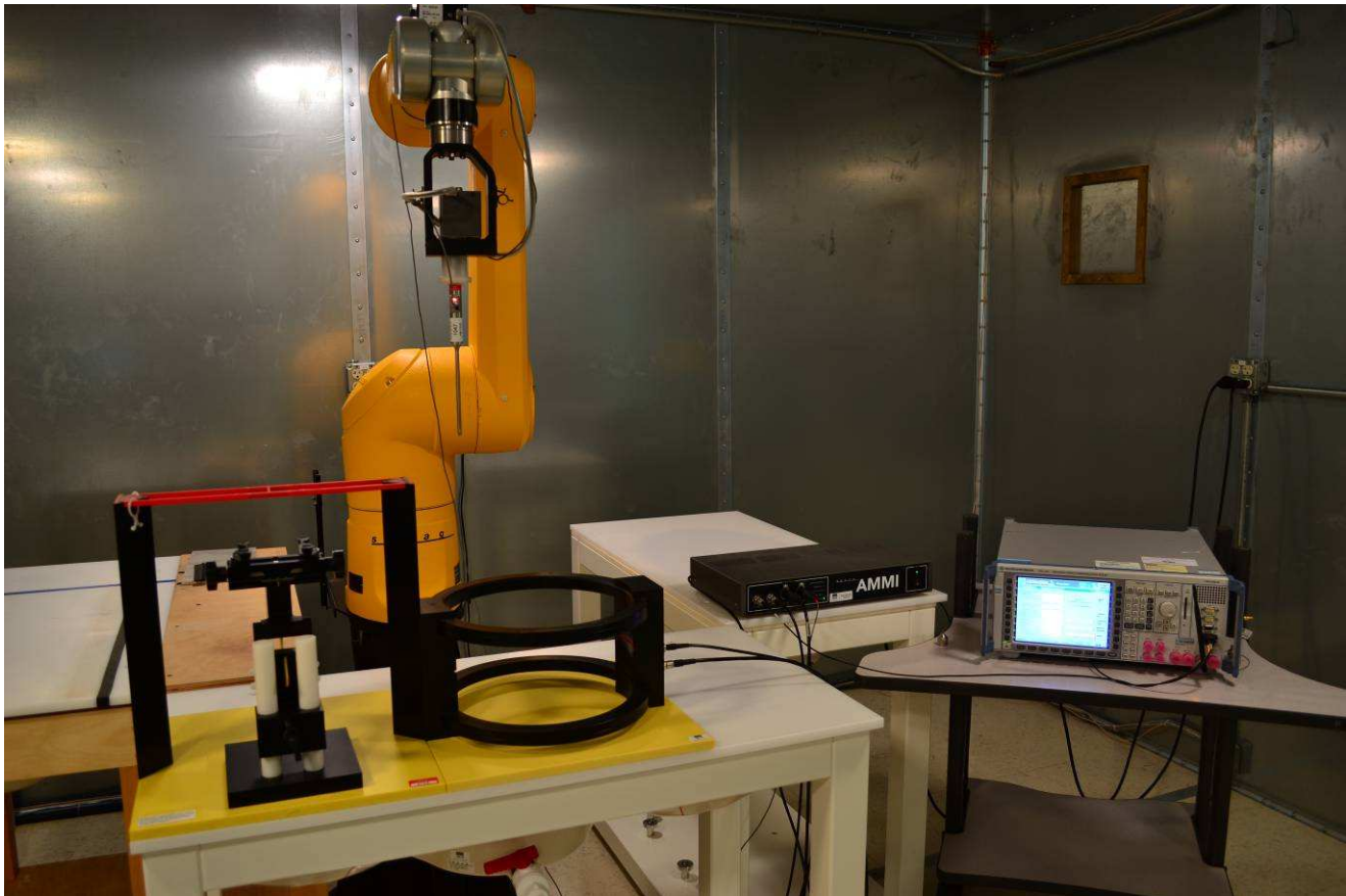
Figure 1: Intertek HAC T-Coil Test Site
