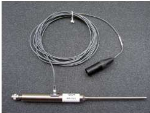
Figure 4: AM1D Probe with probe cable
