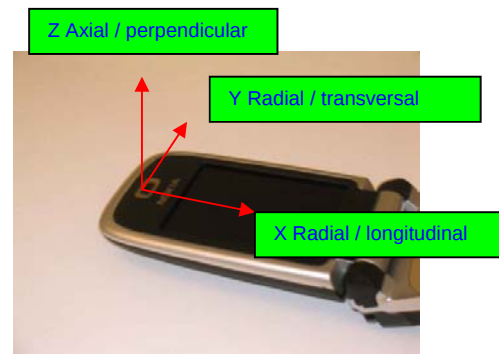
Photo of the device positioned under Test Arch and coordinate system (The EUT in picture is generic phone sample and does not represent the actual equipment under test)
