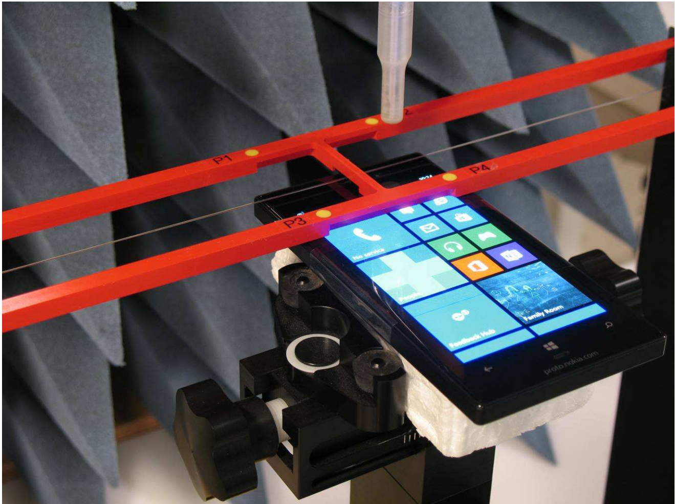
Figure 3: Test Setup Photograph – Near Field Emissions Test
