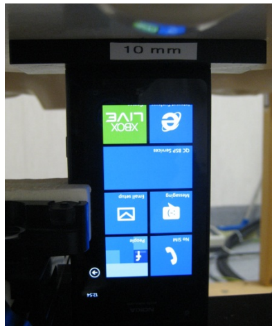
Photo of the device positioned for WR mode measurement – bottom edge facing phantom. The spacer was removed before the start of the measurements.
