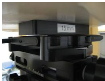
Photo of the device positioned for Body SAR measurement. The spacer was removed for the tests.
