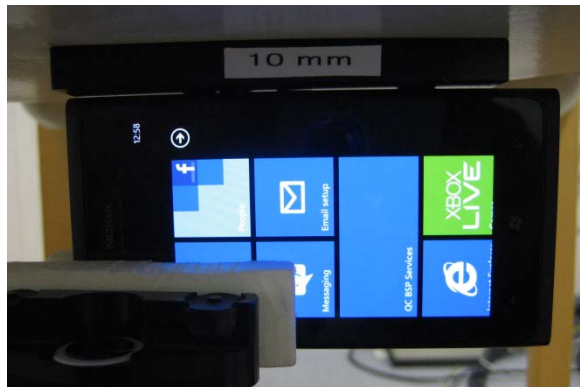
Photo of the device positioned for WR mode measurement – right edge facing phantom. The spacer was removed before the start of the measurements.
