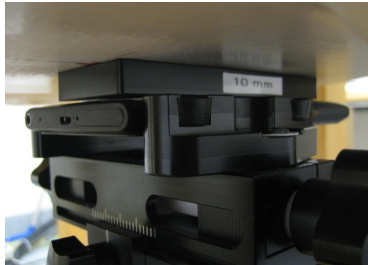
Photo of the device positioned for WR mode measurement – back facing phantom. The spacer was removed before the start of the measurements.
