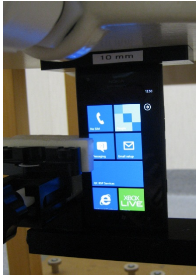
Photo of the device positioned for WR mode measurement – top edge facing phantom. The spacer was removed before the start of the measurements.
