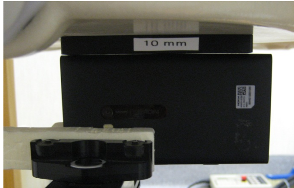
Photo of the device positioned for WR mode measurement – left edge facing phantom. The spacer was removed before the start of the measurements.
