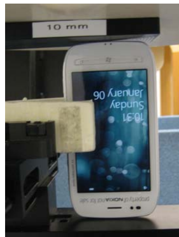
Photo of the device positioned for WR mode measurement – bottom edge facing phantom. The spacer was removed before the start of the measurements.
