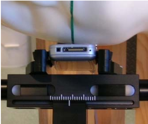
Photo of the device in "cheek" position
