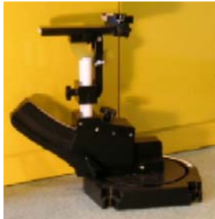
Device holder supplied by SPEAG
