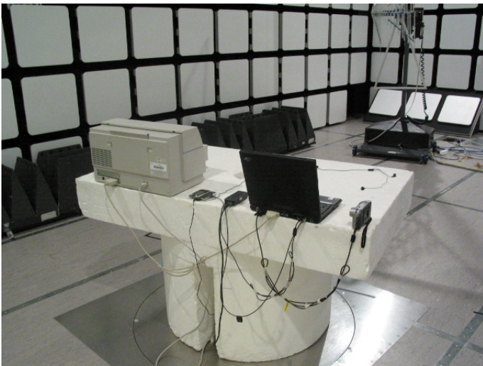
Picture 2 Radiated emission 15B
