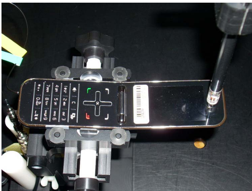
Figure 13-1 Test Setup for Wireless Device
