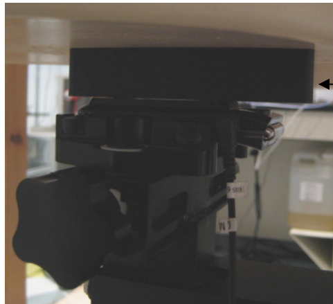
Photo of the device positioned for Body SAR measurement. The spacer was removed for the tests.
