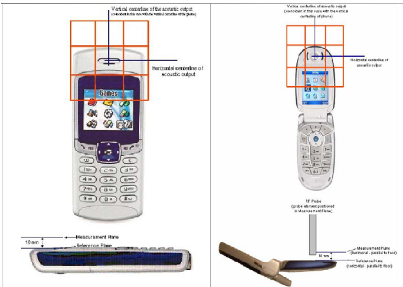
<Figure- 2 > WD reference and plane for T-Coil measurements
