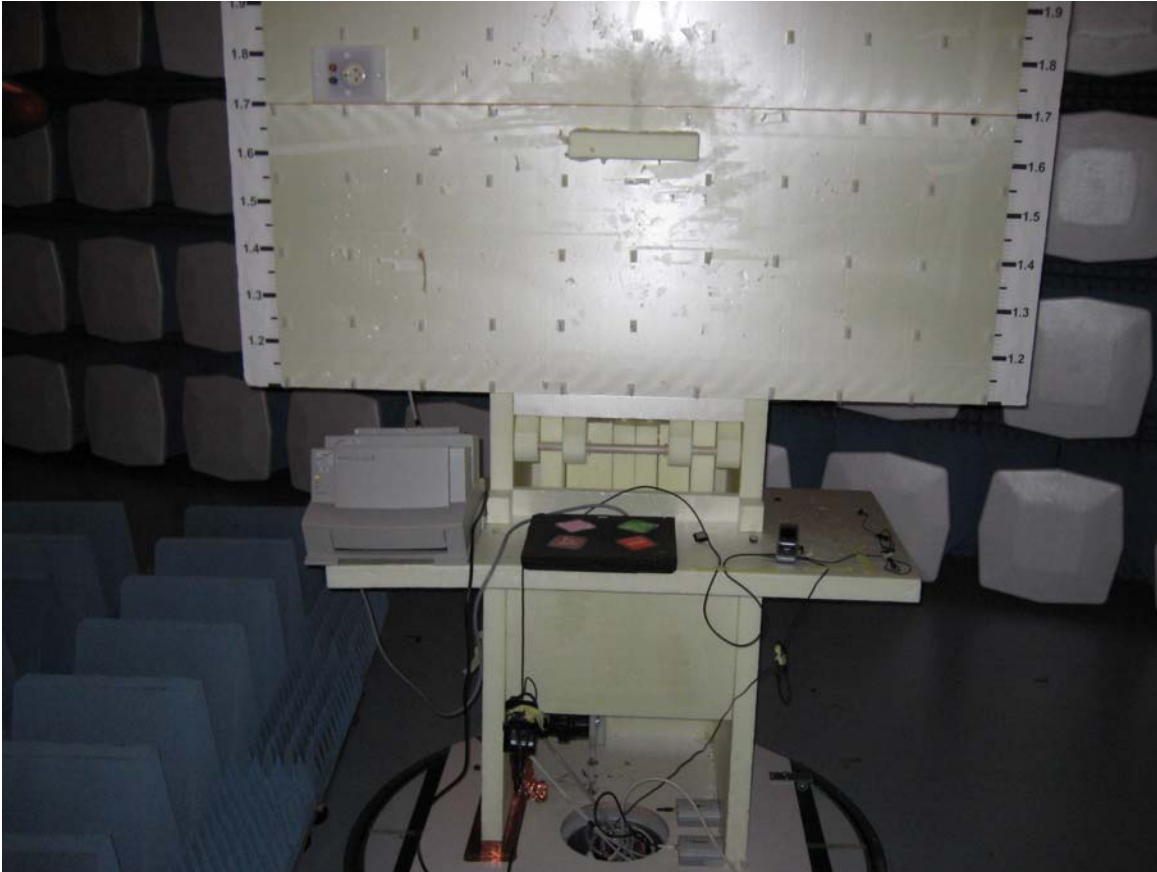
Picture 2 Radiated emission measurement GSM RX/BT TX + Computer peripherals
