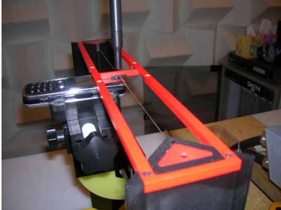
Figure 17-1 Ear Reference Point HAC Phantom Alignment
