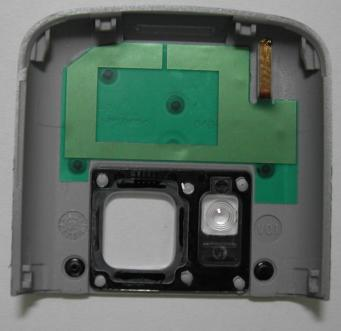
Photo of Internal Antenna of Sample Tested
