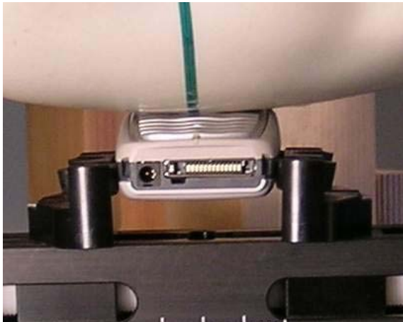
Photo of the device in "cheek" position
