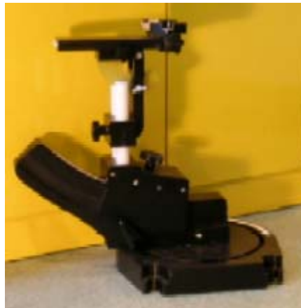
Device holder supplied by SPEAG
