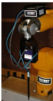
Figure 9 SPEAG Robotic System
