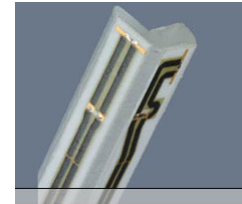
Figure 4 E-field Free-space Probe
