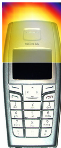
Figure 28 Sample H-field Scan Overlay
