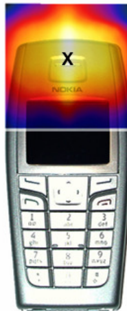
Figure 27 Sample E-field Scan Overlay
