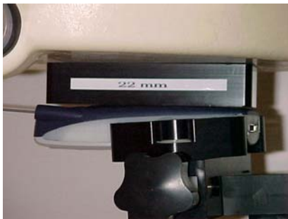
QMNRH-44 with 22 mm distance spacer before measurements
