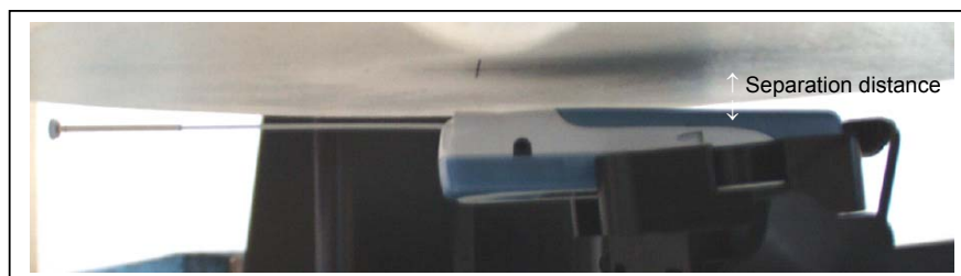
Fig. 5.1.4.1. QMNRH-3P in body position with antenna extended and headset HDB-4 connected.
