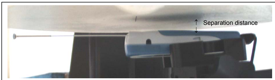
Fig. 5.1.4.1. QMNRH-3DNG in body position with antenna extended and headset HDB-4 connected.
