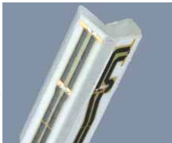
Fig. 5.2 E-field Free-space Probe
