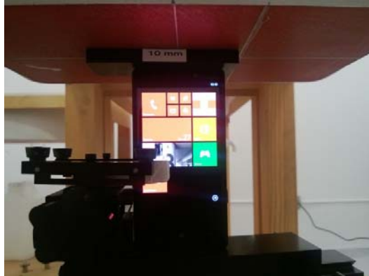
Photo of the device positioned for WR mode measurement – top edge facing phantom. The spacer was removed before the start of the measurements.
