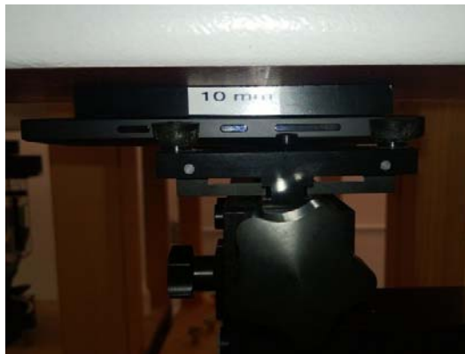
Photo of the device positioned for WR mode measurement – display facing phantom. The spacer was removed before the start of the measurements.
