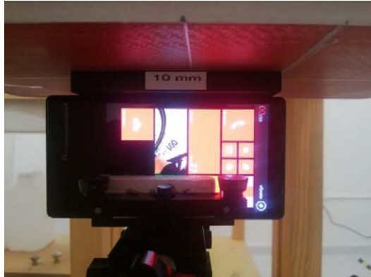
Photo of the device positioned for WR mode measurement – left edge facing phantom. The spacer was removed before the start of the measurements.
