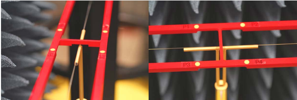
Figure 2: Dipole Mounted under Test Arch
