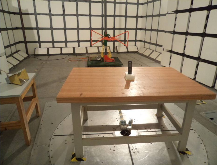
Radiated Emissions View (Below 1 GHz)
