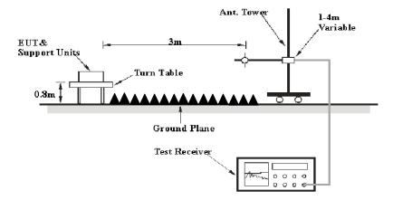
The radiated emission tests were performed in the 3 meters chamber test site, using the setup accordance with the ANSI C63.17 - 2006. The specification used was the FCC 15.209 and FCC 15.319(g) limits.
