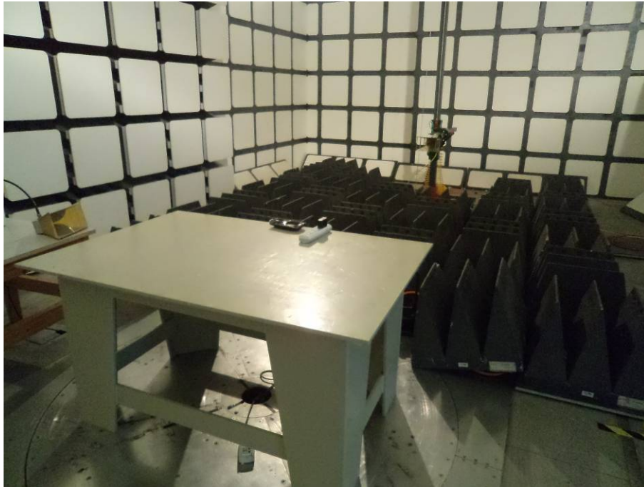
Radiated Emissions - Front View (Above 1 GHz)
