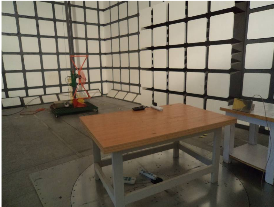
Radiated Emissions - Front View (Below 1 GHz)
