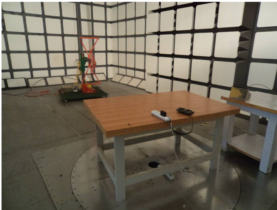
Radiated Emissions - Rear View (Below 1 GHz)
