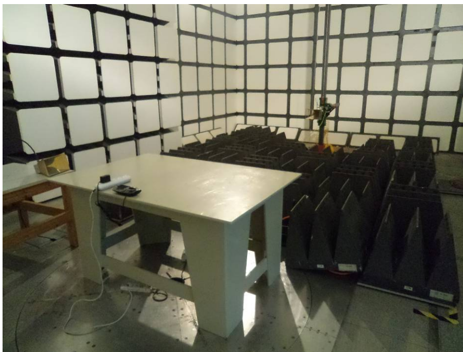
Radiated Emissions - Rear View (Above 1 GHz)
