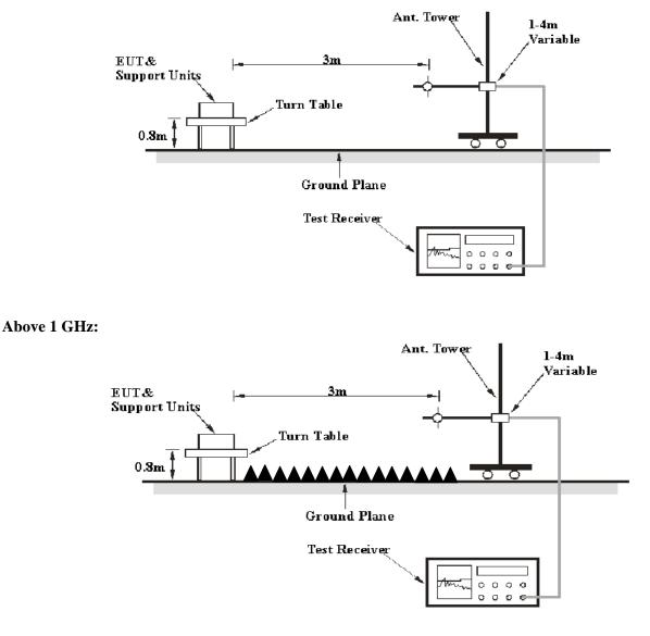
The radiated emission tests were performed in the 3 meters chamber test site, using the setup accordance with the ANSI C63.17 - 2006. The specification used was the FCC 15§ 15.319(g).
