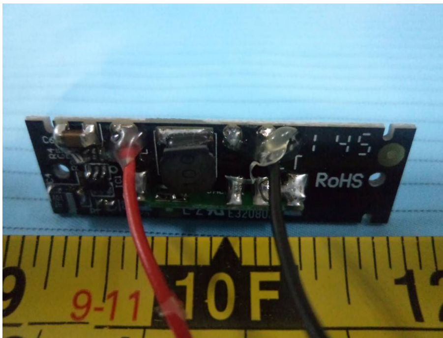
EUT – iPhone Charging Board Bottom View
