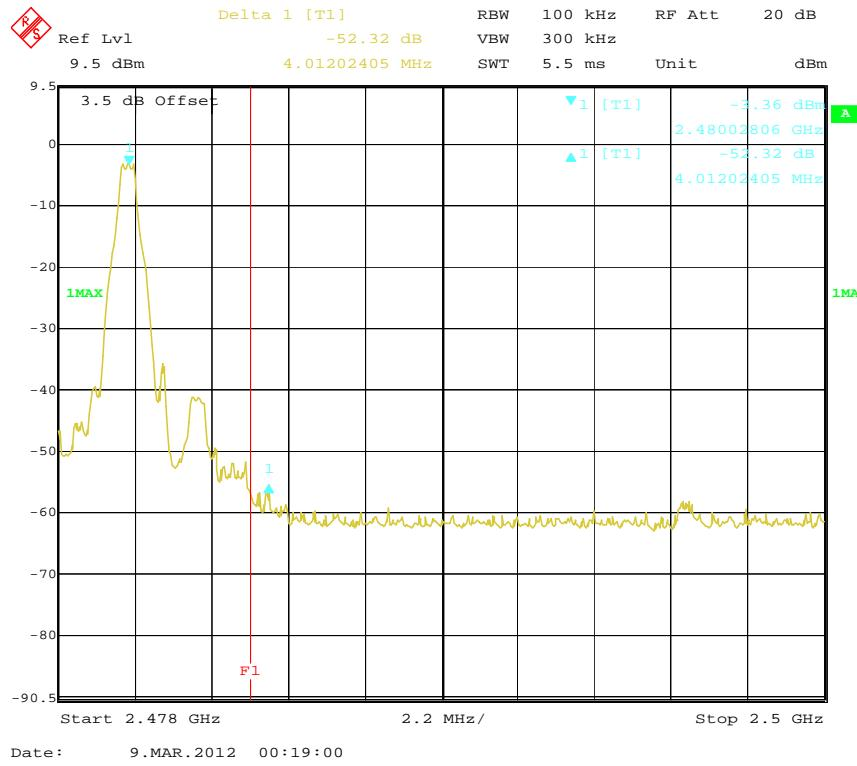
**$\pi/4$ -DQPSK - Band Edge: Left Side**
