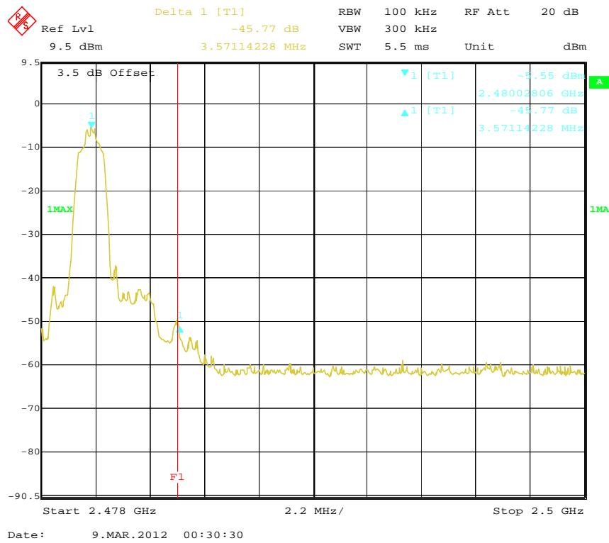
**8DPSK - Band Edge: Left Side**
