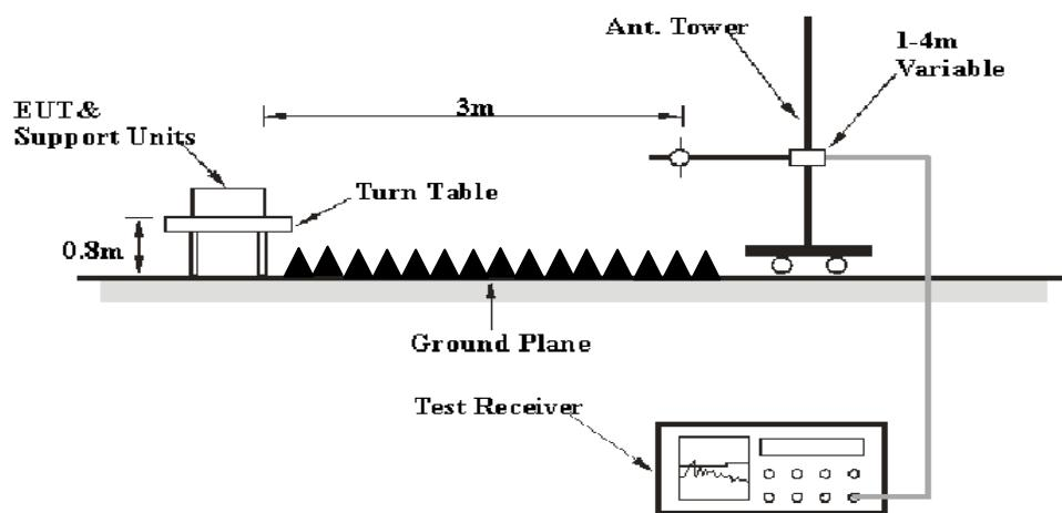
The radiated emission tests were performed in the 3 meters chamber test site, using the setup accordance with the ANSI C63.4-2009. The specification used was the FCC 15.209, and FCC 15.247 limits.
