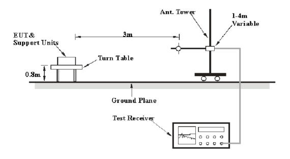
The radiated emission tests were performed in the 3 meters chamber test site, using the setup accordance with the ANSI C63.17 - 2006. The specification used was the FCC 15.209 and FCC 15.319(g) limits.
