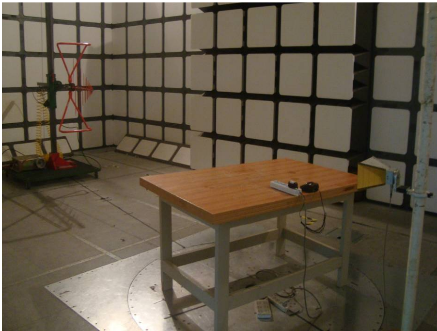
Transmitting: Radiated Emissions - Rear View (Below 1 GHz)
