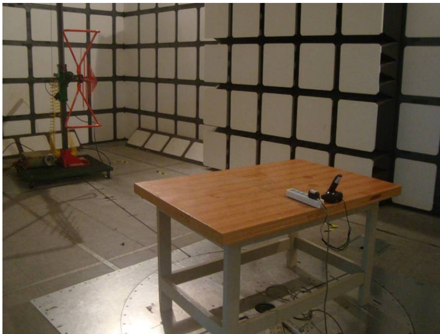
Charging: Radiated Emissions - Rear View (Below 1 GHz)
