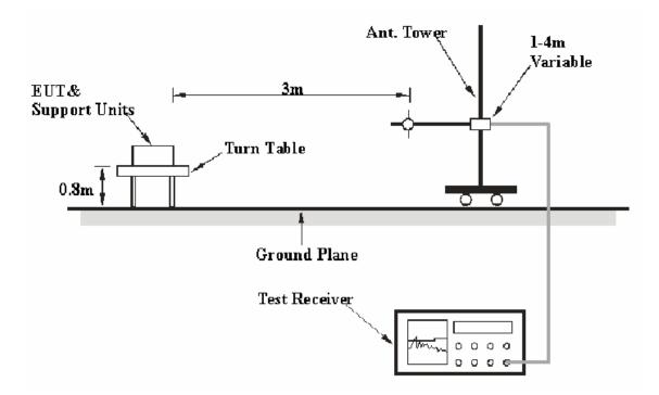
The radiated emission tests were performed in the 3 meters chamber B test site, using the setup accordance with the ANSI C63.17 - 2006. The specification used was the FCC 15 § 15.319(g).
