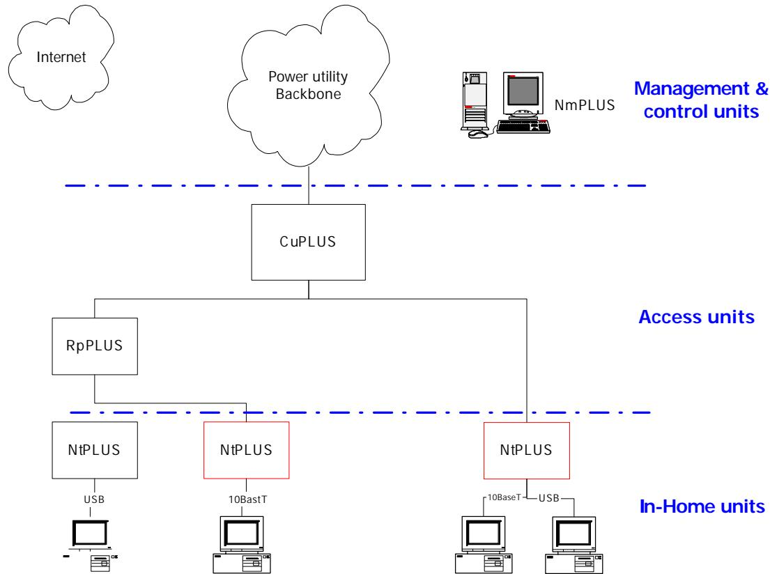
Main.net's Power Line Ultimate System (PLUS) has a unique concept that provides a highly cost-effective telecommunication solution for high-speed transmissions over low and medium voltage power lines.
